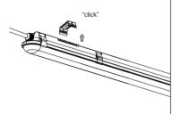
8. Fix the luminaire with the brackets.
