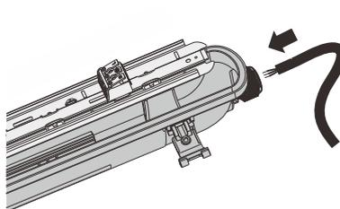
5. Insert the cable through the cable gland
