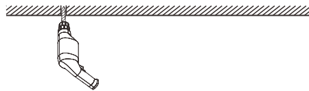
1. Drill a \varnothing 6\text{mm} hole
