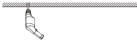
1. Drill a \varnothing 6\text{mm} hole
