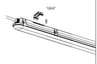
8. Fix the luminaire with the brackets.
